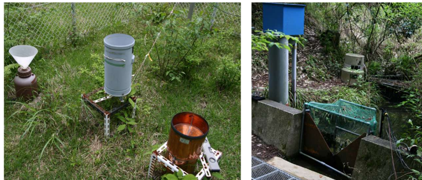
降水量観測（左）・流量観測（量水堰）（右） Pictures of precipitation (left), stream runoff (Weir) (right) observations
