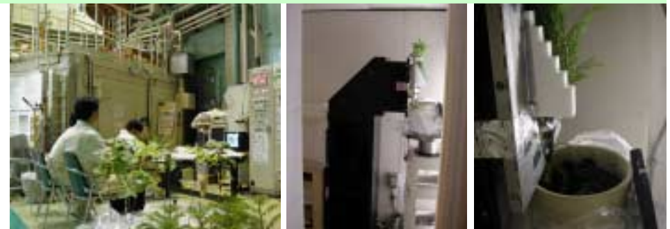
Fig.4 Thermal neutron radiography facility of JRR-3M Left, whole view; Center, inside the irradiation chamber; Right: seedling and Teflon standard fixed on an aluminum cassette, where an X-ray film (Kodak SR) and a gadolinium n / \gamma converter (25mm in thickness) were sealed in vacuum.
